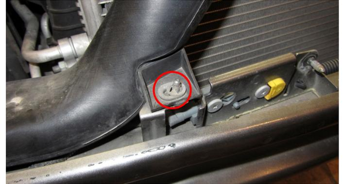
10. Remove the air guide (1.) from the top of the intercooler by pulling it upwards. Remove the 2pcs Torx T25 screws (2.) that attaches the AC condenser to the intercooler.
