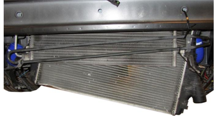
19. To install the intercooler on a 4 cylinder model 9-3 the lower brackets needs to be removed. Drill the 2pcs of rivets on each bracket heads using a 8mm drill and drill only about 3mm (1/8") deep. Take care to not drill too deep. If you drill about 10mm deep you might cause a leak in the core. When the rivets heads are drilled according to this, just bend the brackets loose.
