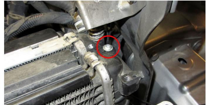
18. Remove the intercooler by lifting it up from the radiator slots and then carefully remove the intercooler downwards starting with the left hand side and then the rest of it according to picture.
