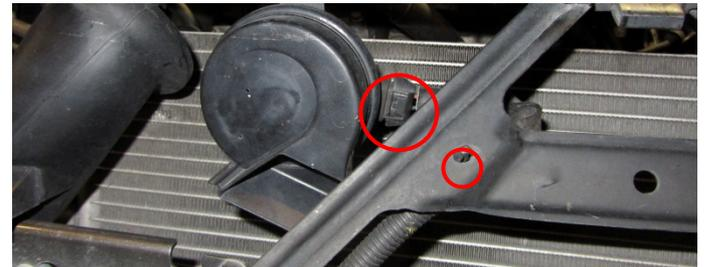
8. Remove the radiator support by removing 8pcs of 10mm (on facelift 6pcs) hex head screws on top of it and 2pcs of 10mm hex head screws in the bottom of the cross member.
