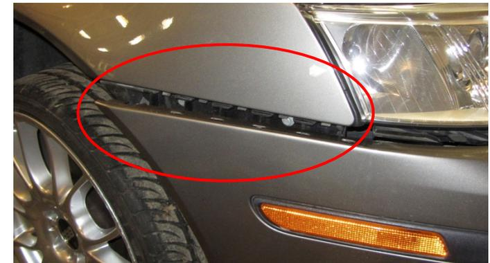
6. Remove the headlights by removing 3pcs of 10mm (on facelift 2pcs 10mm & 1pc 7mm) hex screws on each headlight and then pull/lift forward so you can disconnect the electrical connector from the headlight and then remove headlight from vehicle.
